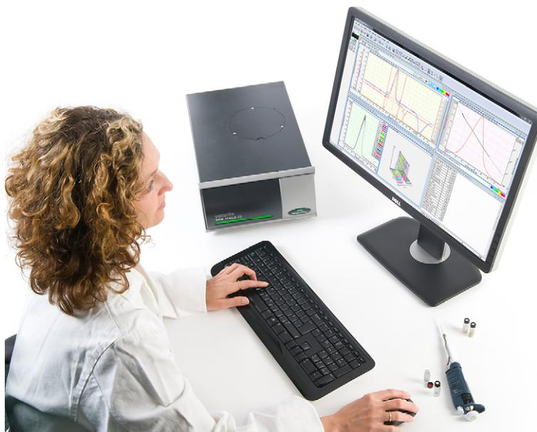
The SEC-MALS 20 is a modular detector that can easily be used with any existing SEC system, adding the power of light scattering detection for molecular weight and size measurements. It can also be purchased as part of a complete system package.
