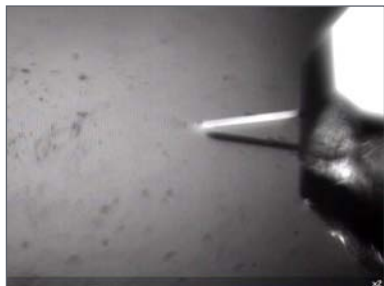
Simultaneous side view image of the same cantilever and sample. Availability of side view is ideal during a first coarse approach.
